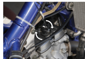
2/4 stroke install: Wrap pickup wire around head of coil
