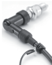
2/4 stroke install: Wrap pickup wire around spark plug lead.
